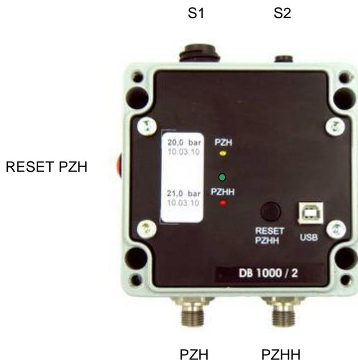
The electronic pressure limiter is supplied in a metal-clad aluminum moulded housing (IP 65). After unscrewing the lid the drilled holes (hole diameter 5mm) can be seen which allow you to fasten the DB1000/2 in place on the unit. Data regarding permissible vibration strain can be found under point 6.
