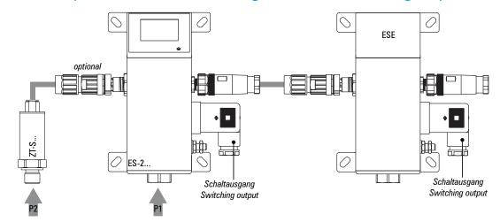
Apart from additional measuring channels, more switching contacts are added by means of an extension unit (ESE). This makes it possible to set up a shared safety chain, e.g. of several pressure transmitters and switching outputs.
