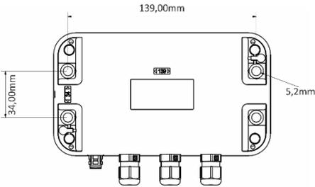
**3:** Mount the unit at a suitable place on the wall by inserting the screws through the holes provided in the housing and fastening the screws.
