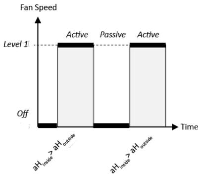
The KST-20 Vento works as an intelligent power switch and controls the active and passive phases of 1-stage fans.
