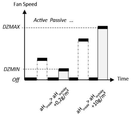
Speed-controlled fans are operated within the two adjustable limits "minimum speed" (DZMIN) and "maximum speed" (DZMAX). The speed corresponds to the control voltage in percent. The lower limit DZMIN starts by default at  $aH_{inside} > aH_{outside} + 0,2g/m^3$ . The upper speed limit DZMAX is activated at  $aH_{inside} > aH_{outside} + 10g/m^3$ . In between, the output of the control voltage is linear.
