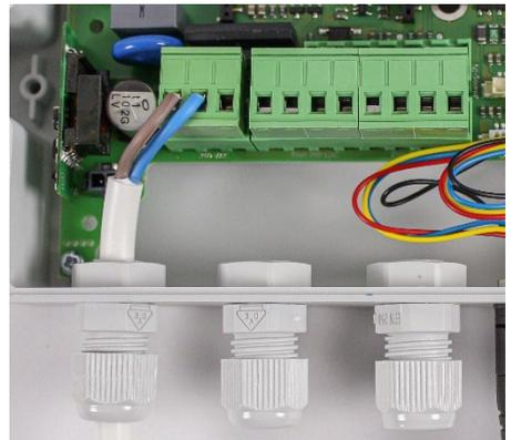
**6:** When all electrical cables are correctly connected, place the housing cover (2) back onto the lower part of the housing (3) and fasten it by loosening the screws.
