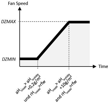
Basic ventilation only continues with DZMIN until the desired humidity is reached or the absolute humidity inside is lower than the absolute humidity outside.
